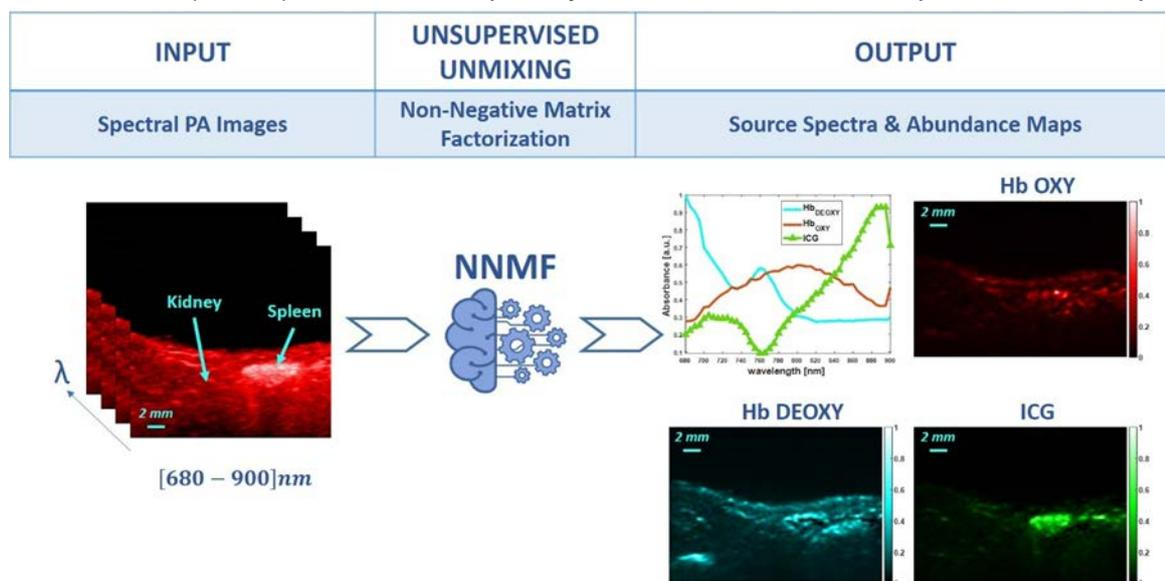
Fig. 2: Schematic chart of the NNMF-based unmixing approach to detect endogenous chromophores such as Oxygenated (Hb Oxy) / Deoxygenated (Hb Deoxy) Haemoglobin and exogenous contrast agents such as ICG, after intravenous injection in a CD1 healthy mouse model. ESR 15 (VSI) published in V. Grasso et al.: An Automatic Unmixing Approach to Detect Tissue Chromophores from Multispectral Photoacoustic Imaging. Sensors 2020, 20(11), 3235; <https://doi.org/10.3390/s20113235>
