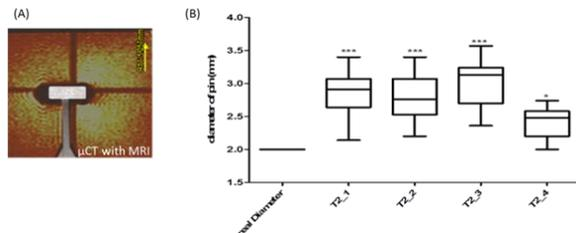
Fig. 1 (A) combination of  $\mu$ CT and MRI of the Mg pin showing the artefacts in MRI around the edges of the pin. (B) Plot of the Mg pin size in after different changes in sequences to reduce the artefacts. (ESR 5, MHH)
